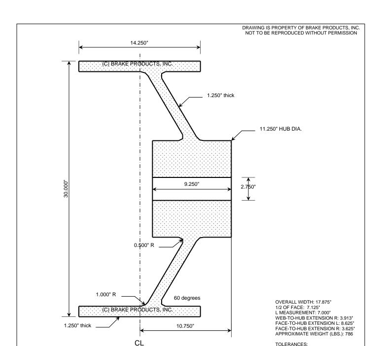
TOLERANCES: WHEEL DIAMETER: +0.005"/-0.000" BORE DIAMETER: +0.000"/-0.001"
